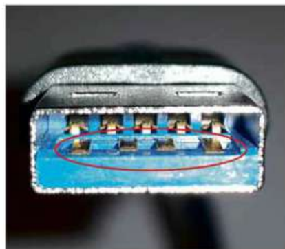
USB adapters have four primary metal contacts – two for power, the other two for data
