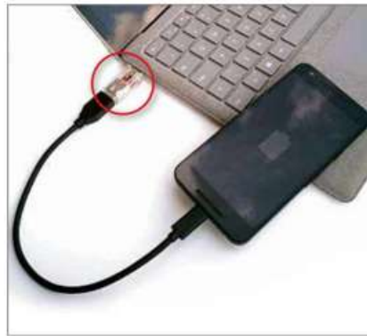
A USB condom sits between your USB cable and the device you're plugging into
